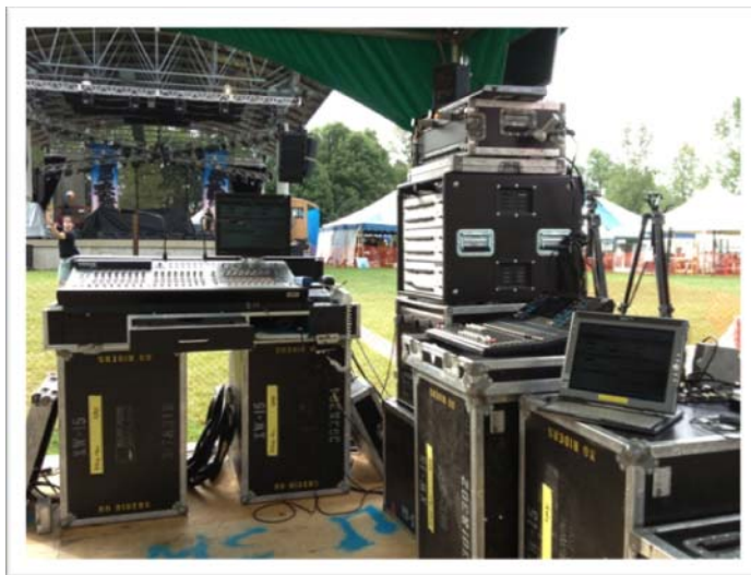
A: Main Stage FOH set-up including Digidesign SC-48 and Yamaha LS9 consoles, along with SMAART and Tablet controls.
